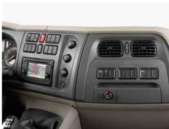
**PRACTICAL** The new dashboard has a 12-volt socket and a double DIN box that is suitable, among others, for the Truck Navigation Radio. In the console over the engine tunnel, there is a USB connector and a 24-volt socket. Ideal for connecting a smartphone, tablet, laptop or MP3 player.
