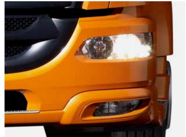
**SAFE** The lighting of the LF contributes to its visibility and safety. The headlight units are optionally available with daytime running lights. They are made of unbreakable Lexan, just as the optional fog lights and cornering lights. These cornering lights turn with the steering and shine in the direction of travel. Convenient and safe when turning or manoeuvring and even less chance of damage.
