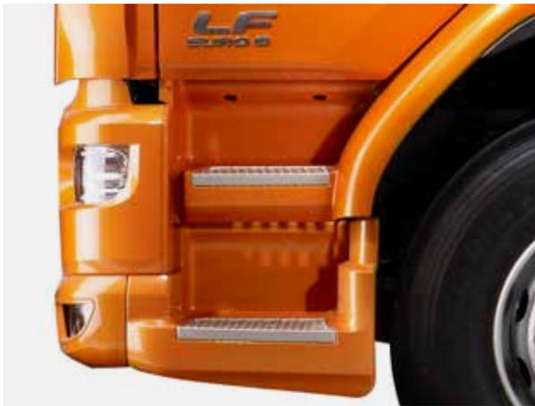
**PRACTICAL** Intensive distribution transport means a lot of climbing in and out the cab. That's why the new LF offers maximum accessibility. Thanks to doors that open 90 degrees and a very low floor height of 89, 98 or 111 cm, depending on the version. Wide non-slip steps, carefully positioned handgrips and convenient step courtesy lights make comfort for driver and co-driver complete.
